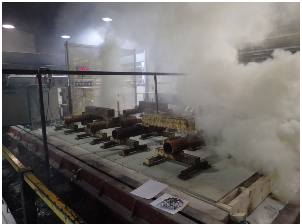
The unexposed face of the assembly after 90 minutes of testing
