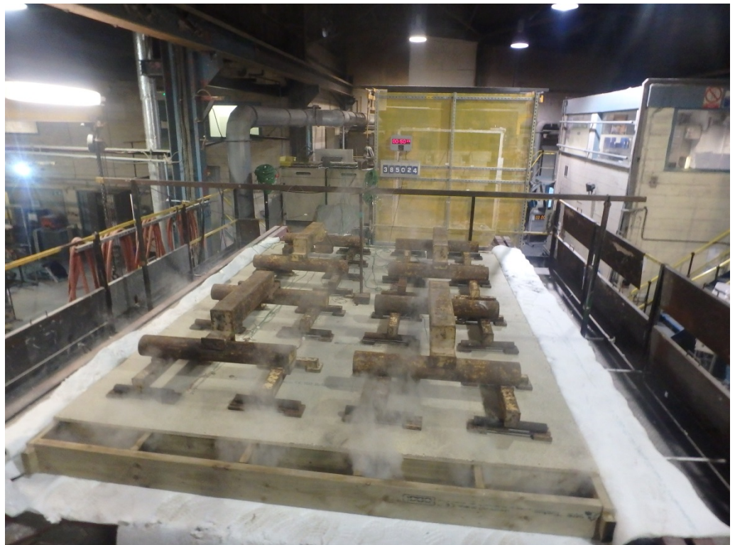
The unexposed surface of the assembly after a test duration of 50 minutes
