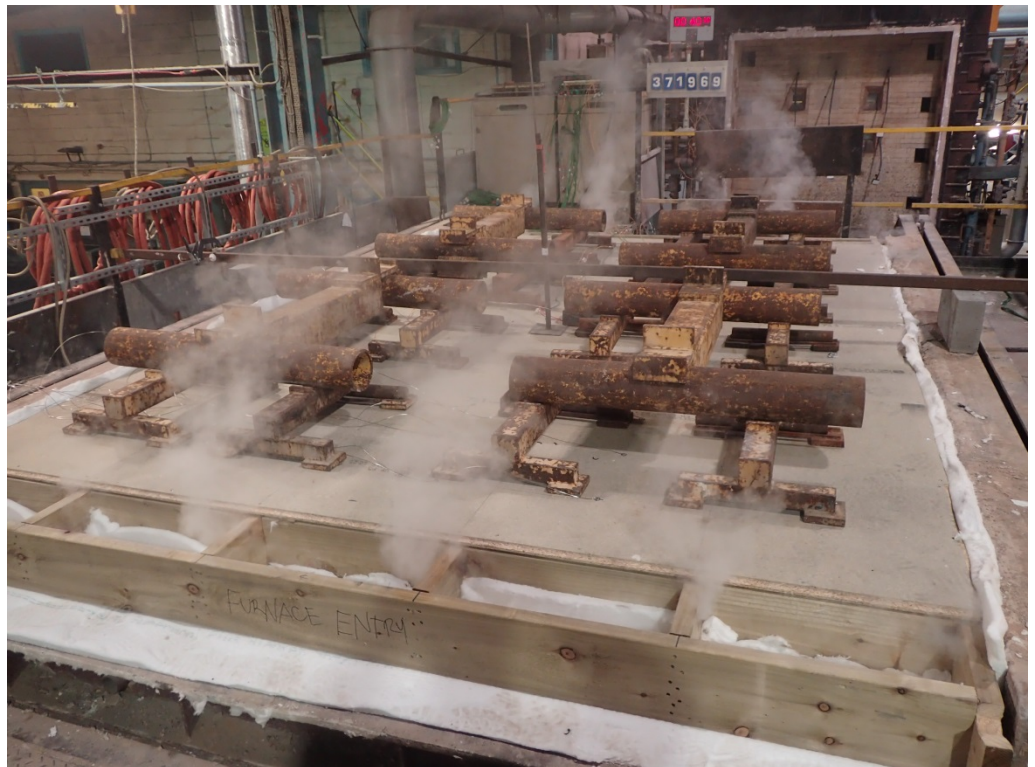
The unexposed face of the assembly after 40 minutes of testing
