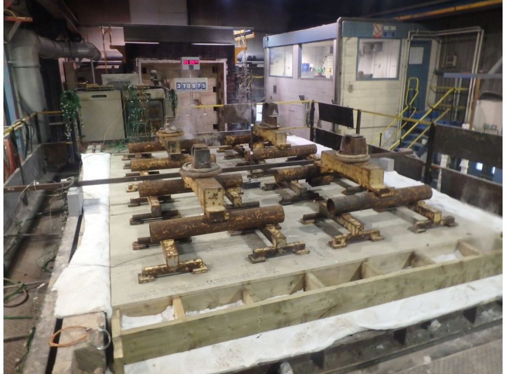
The unexposed face of the assembly after 60 minutes of testing
