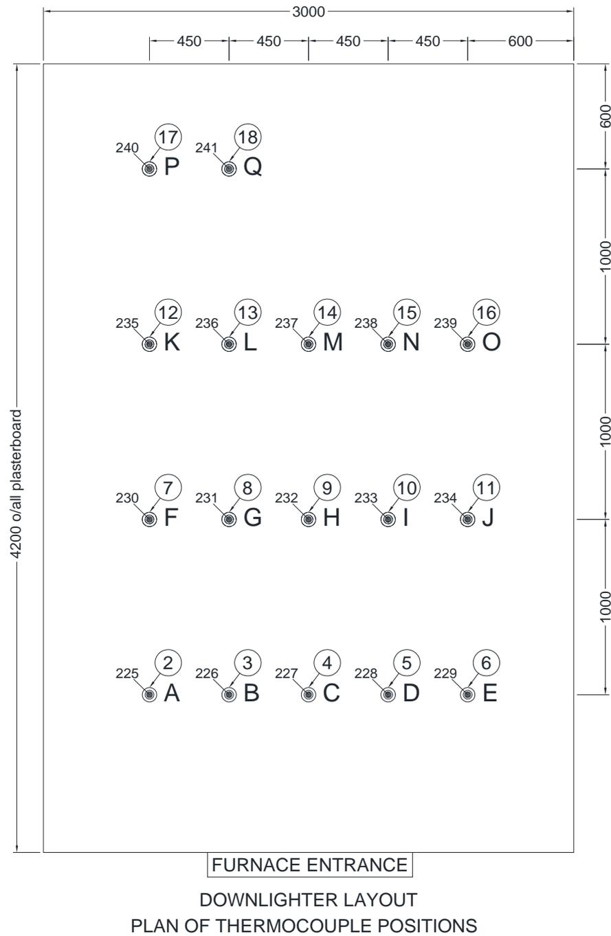
• Mineral insulated thermocouples at mid-cavity height
