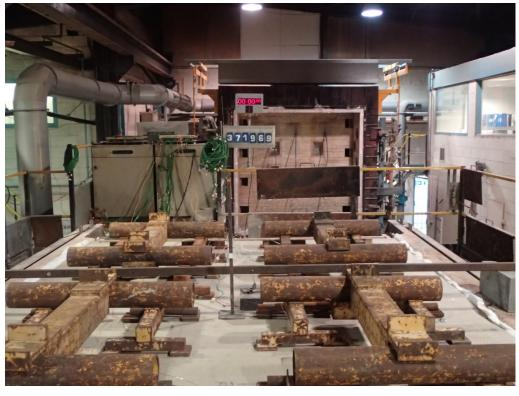
The unexposed face of the assembly after 20 minutes of testing
