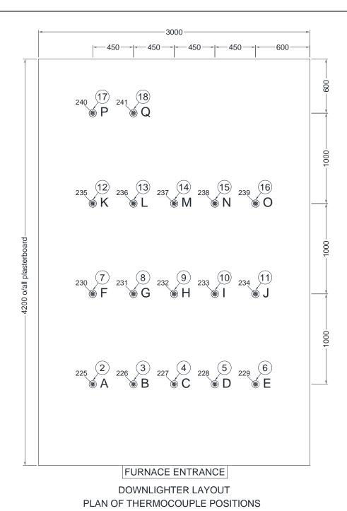
• Mineral insulated thermocouples at mid-cavity height
