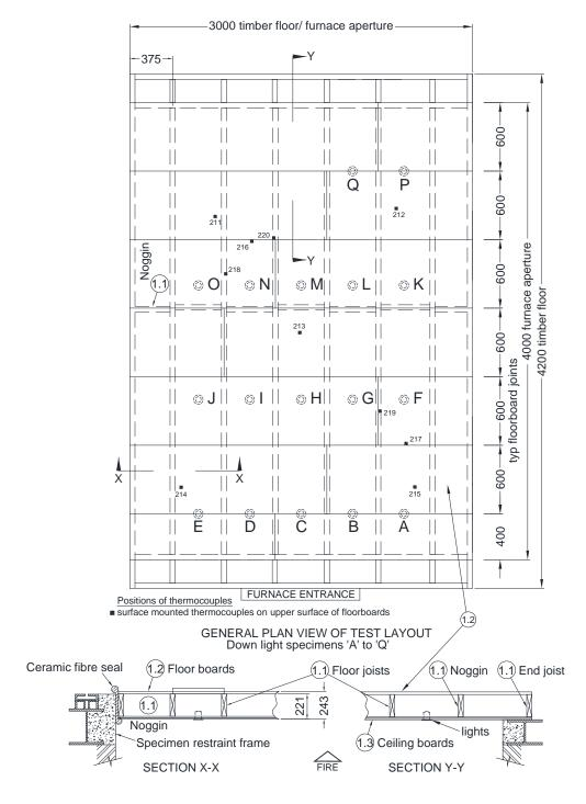
Figure 2 - Details of Downlighter Positions
