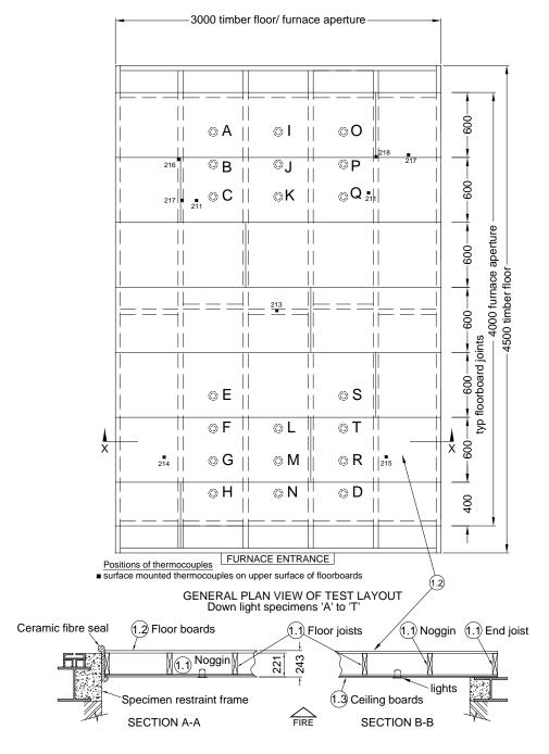
Figure 2 – Details of Downlighter Positions
