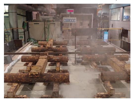
The unexposed face of the assembly after 40 minutes of testing
