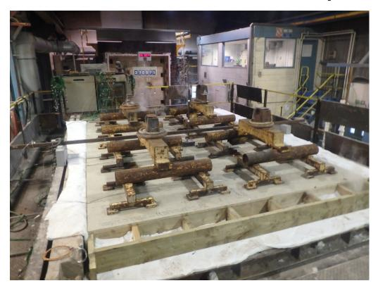
The exposed face of the assembly after a test duration of 60 minutes
