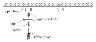
C. Open the end with input mask according picture 1 & picture 2, then open corresponding preset line hole according to th input cord loaction, pictures 3, and fix the cord clip.
