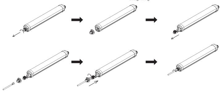
Make a right position and screw hole on the ceiling, screw the clip on
