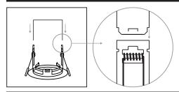
If insulation needs to be laid on top of the Evofire product, an insulation guard is required. To install the insulation guard, push tabs into the Evofire body until they lock into place.
