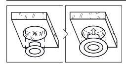
If the hole is greater than maximum cut-out size, an adapter can be used to increase the size of the product.
