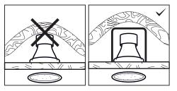
The product should not be covered with insulation material unless using with an optional insulation guard.
