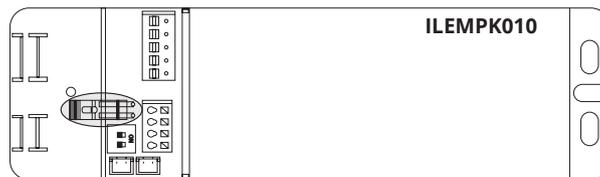
The function of the system reset is to ensure that the convertor is fully disconnected from the LED lights.
