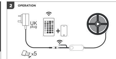
Connect the power supply, controller, and light strip. Then connect it to the AC power grid.
