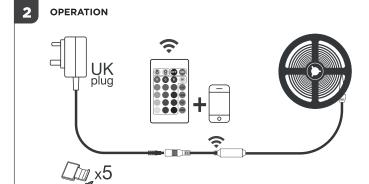
Connect the power supply, controller, and light strip. Then connect it to the AC power grid.
