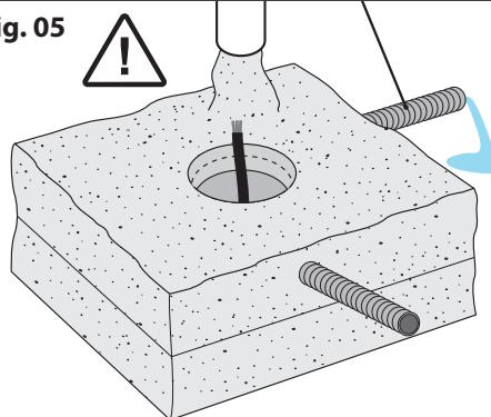
Tube for drainage for concrete applications
