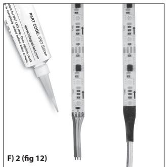
**⚠ CAUTION :** When applying connection wires to the strip, ensure that the correct polarity is observed. Always observe polarity for 12V connections to control unit, please pay attention on the direction of arrow (➡) on strip, positive: red cable (+) to DC+, DIN: white cable to DATA, and (-) yellow cable to GND. (See fig 1. This is based on using Integral controller ILRC013. It may vary depending on the controller).
